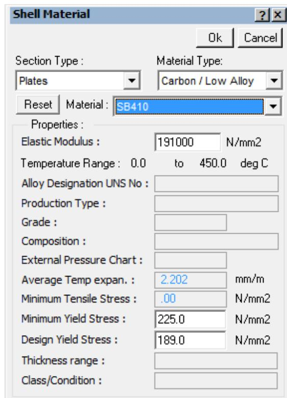
Set “Section Type” = (Plates), and “Material” = (SB410). Some values will be automatically set on the dialog after these selections are made. Now press the <Ok> button and then enter the other data on the Shell tab as follows:
