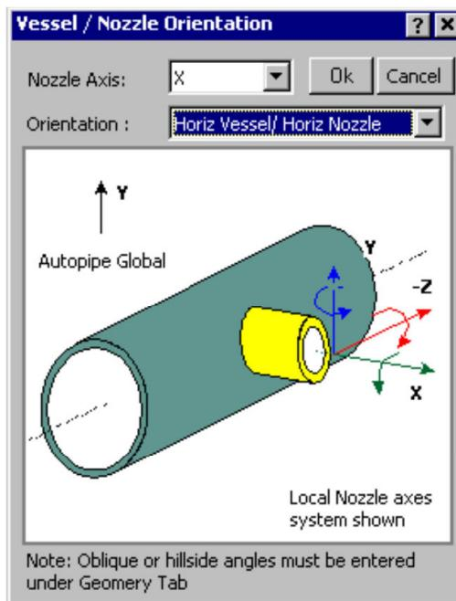
Select the direction of the nozzle and the Vessel, and then press the <Ok> button. All of the Anchor loads of AutoPIPE will automatically be imported into AutoPIPE Nozzle. This data can be viewed on the **Load** tab. It should be noted that the coordinate system of both AutoPIPE Nozzle and AutoPIPE may be different; the program will automatically perform coordinate transformation when the data is imported.
