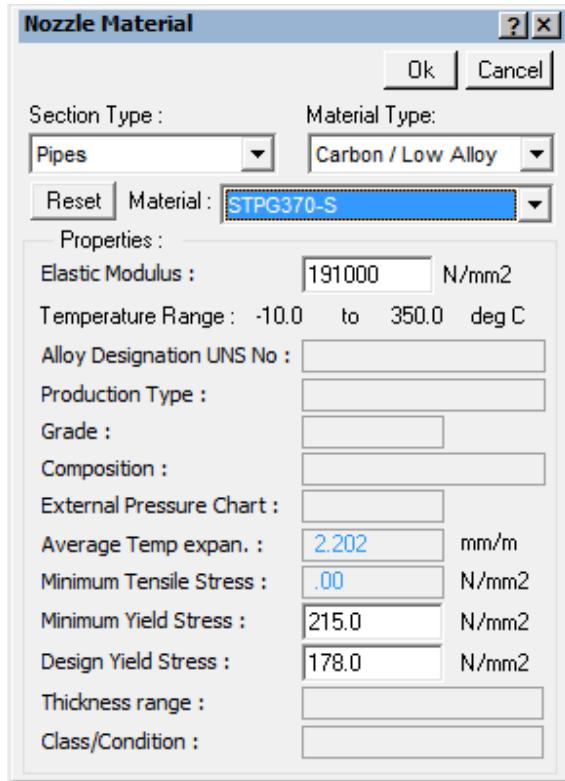
Select the “**Section Type**” = (**Pipes**), select the (**STPG370-S**) from Material drop down listing and then press the <Ok> button. Some values will be automatically set on the dialog after these selections are made. Now press the <Ok> button and then enter the other data on the Nozzle tab as follows:
