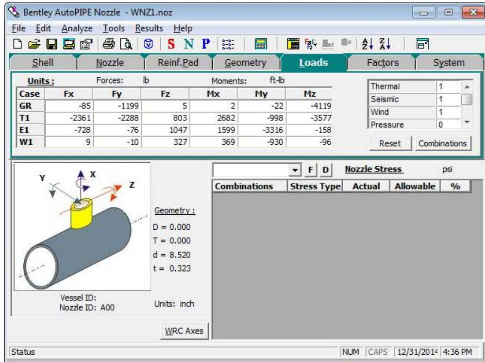
After importing the nozzle load from AutoPIPE continue filling out the other tabs with data as needed before running an analysis in AutoPIPE Nozzle.
