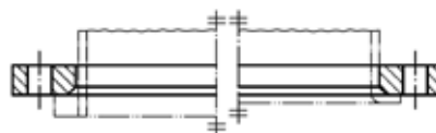
Type 02 Loose plate flange with weld-on collar (see type 32) or lapped pipe end (see type 33)
