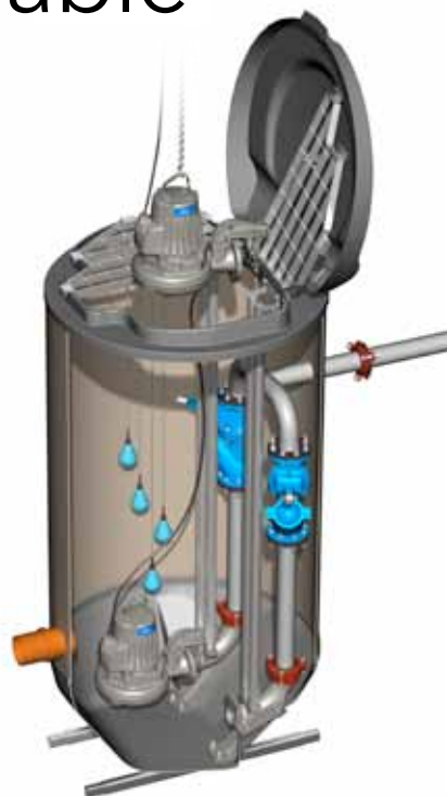
In a two-pump station, four level regulators are generally used. One is positioned at the stop level, one at each pump's start level, and the fourth regulator is used to trigger a high level alarm.
